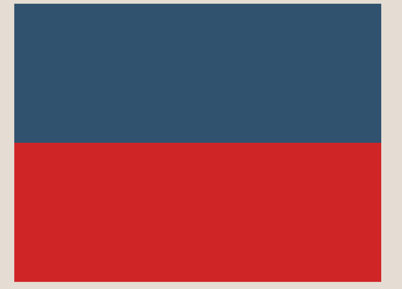
ECHO ALTERING COURSE TO STARBOARD
